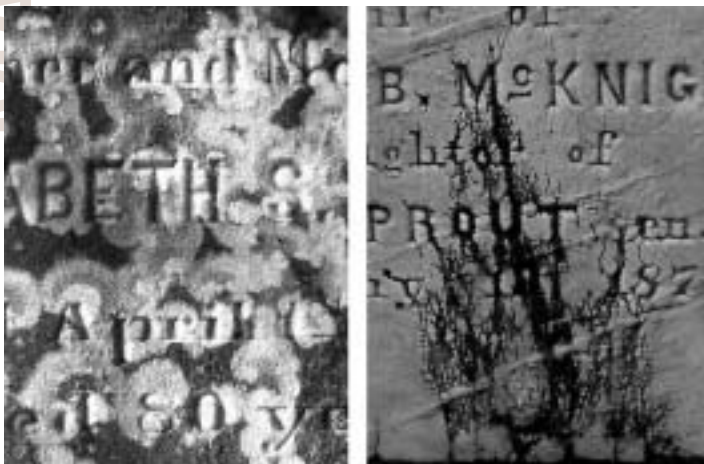
Bacterial and fungal decay of marble headstones
