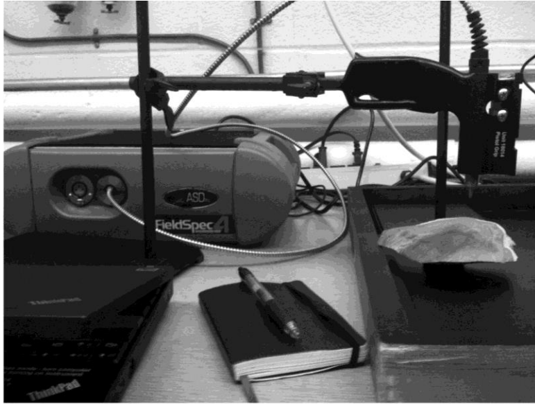
Figure 3. An ASD Inc. FieldSpec® spectrometer used to obtain spectra in the visible and near-infrared regions.
