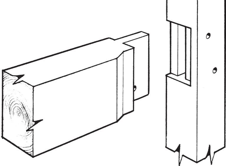
*Paired Through Mortise and Tenon (Fig. 8).* In frames with larger members, paired or twin tenons were occasionally used. Such a configuration will likely outperform a simple mortise and tenon, with reduced tendency for pin shear and mortise-face splitout. However, the advantage must be judged against the substantial additional work in the cutting of the joint. Paired tenons are sometimes found in mill structures, barns and large wooden machines like cider presses.
