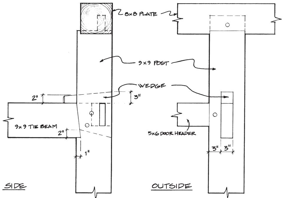
Figs. 11 and 12. Below and below right, assembled and exploded views of a wedged dovetail through mortise and tenon with dovetailed housing, as found in a 28x34-ft., three-bay side entrance barn in East Chatham, New York, probably dating from the second half of the 18th century. This unique joint has exceptional tensile strength.
