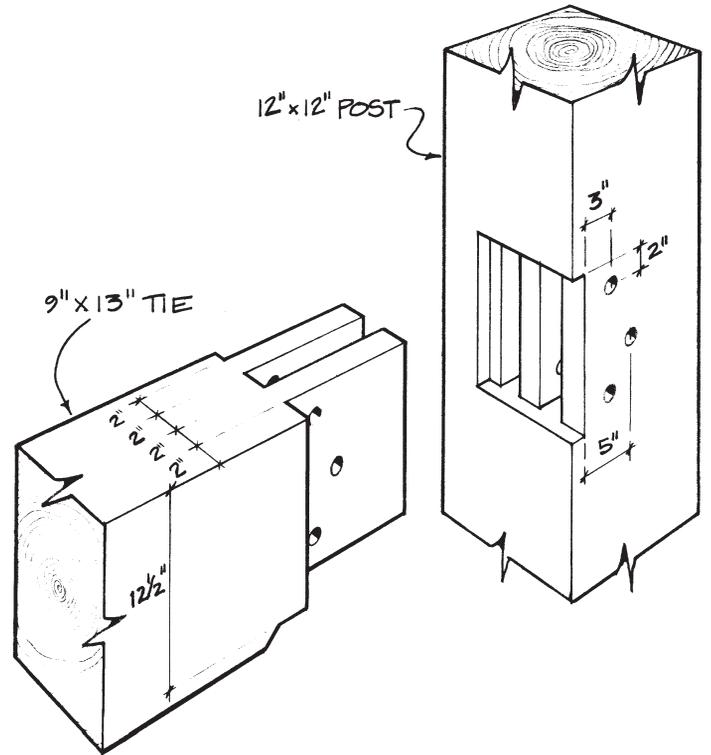
*Fig. 8. Paired or twinned through mortise and tenon as found in a ca. 1840 barn in Middleburg, New York. The joint is housed flush with one side. As is typical of square rule structures, the tie beams are reduced to a consistent depth (here 12 1/2 in.) at the joint. This rugged connection has well resisted the forces in the 50-ft.-wide barn.*
