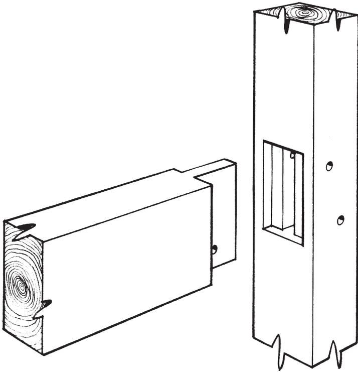
*Fig. 6. In a blind-housed through mortise and tenon, the tie beam may be flush with one side or centered as shown. The uninterrupted long grain flanking the joint on the post resists breaking at the joint and mortise face splitout.*
