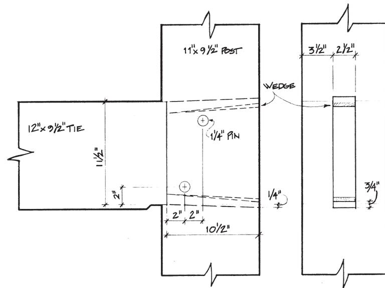
*Fig. 13. This kerf-wedged dovetail through mortise and tenon joint is found in the upper floors (after 1810) of the Machine Shop at Hancock Shaker Village, Hancock, Massachusetts. It was used for both the tying joints and the queenpost trusses. This joint is much more common in furniture than in framing. Because of shrinkage in the height of the tenon, the wedges are loose, indicating that the pins are carrying the load.*
