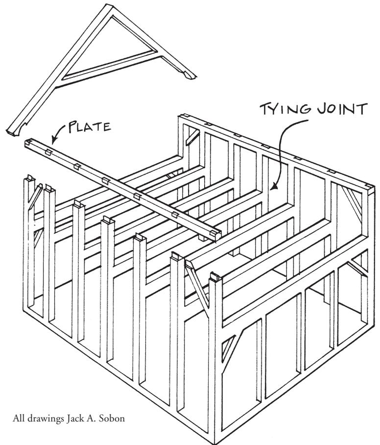
*Fig. 1. In the typical New York State timber-framed Dutch house, the plate is 3 to 4 ft. above the second floor. The closely spaced H-bents, typically 3 to 5 ft. on center, illustrate the tie-below-plate condition.*
