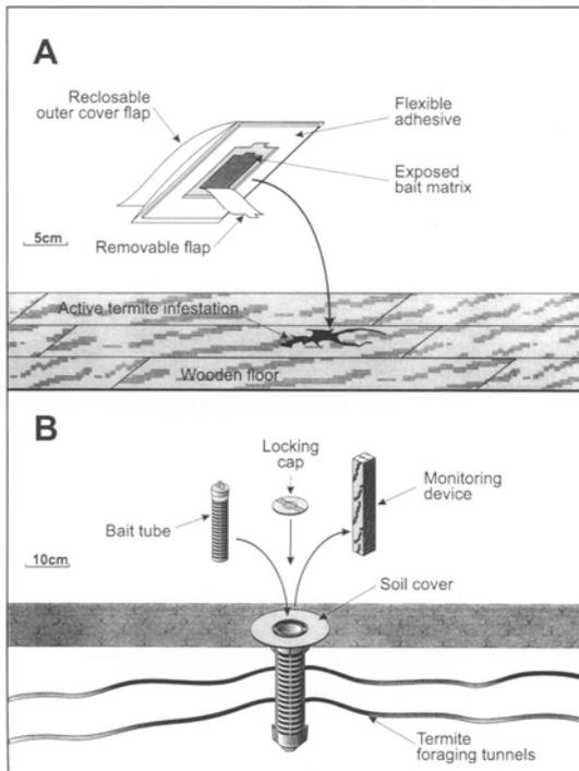
Figure 3. Above-ground bait stations consisting of a flexible laminated pouch containing 15g of 0.5% hexaflumuron bait (A) were placed directly over active infestations of *C. formosanus* in the wooden floors of the Bust Gallery of the Presbytere and the second floor of the Creole House. In-ground (Sentricon) stations were placed in the soil of the Creole House courtyard to detect termites and deliver hexaflumuron baits (B).
